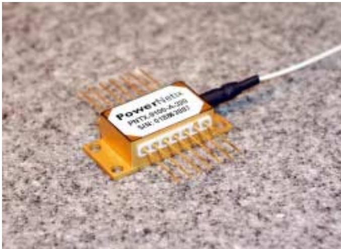
The 9100 Series 980 nm pump module from PowerNetix is a high power, low-profile, 14-pin butterfly package capable of delivering up to 350 mW of fiber-coupled power.
