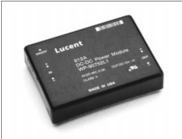
The 912A Power Module uses advanced, surface-mount technology.
