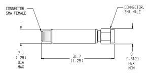
NOTE: All dimensions are given in mm (inches) and are maximum, unless otherwise specified.
