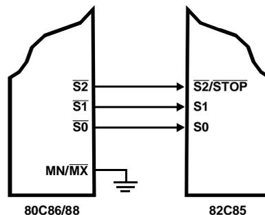
FIGURE 3. 82C85 STOP CONTROL USING 80C86/88 MAXIMUM MODE STATUS LINES
