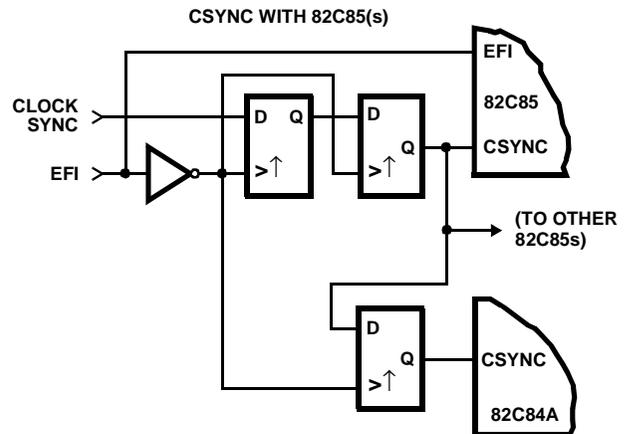
FIGURE 6. 82C85 AND 82C84A CSYNC SYNCHRONIZATION METHODS
