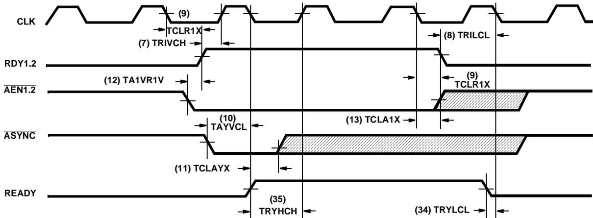
FIGURE 8. WAVEFORMS FOR READY SIGNALS (FOR ASYNCHRONOUS DEVICES)
