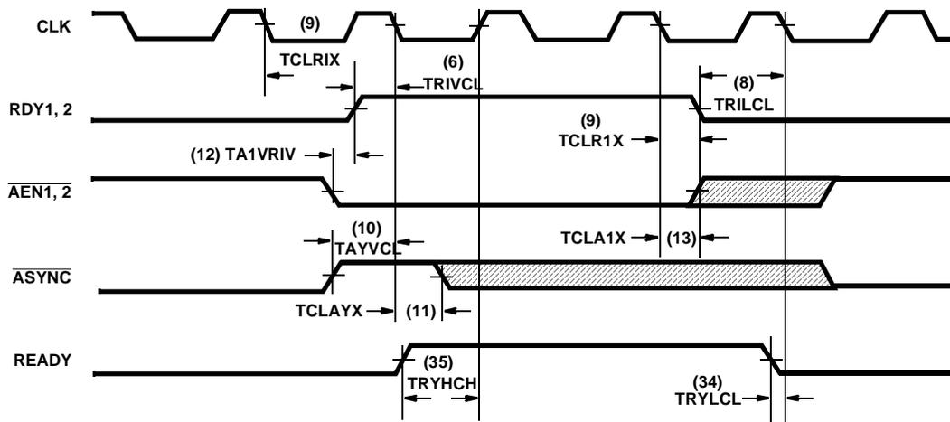
FIGURE 9. WAVEFORMS FOR READY SIGNALS (FOR SYNCHRONOUS DEVICES)
