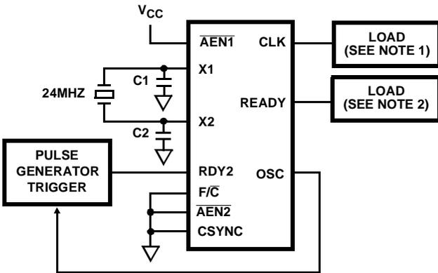
**TRYLCL, TRYHCH LOAD CIRCUIT (USING EFI)**
