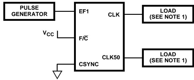
**TRYLCL, TRYHCH LOAD CIRCUIT (USING X1, X2)**
