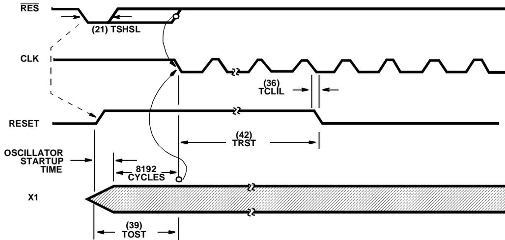
FIGURE 14. RESET TIMING (OSCILLATOR STOPPED,  $F/\bar{C}$  LOW)
