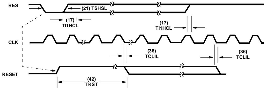
FIGURE 13. RESET TIMING (CLK RUNNING WITH  $F/\bar{C}$  LOW-OSC MODE)
