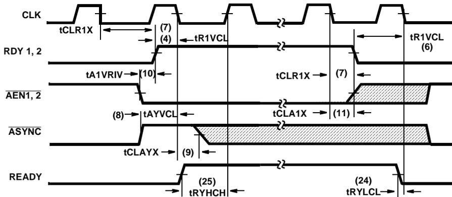
FIGURE 4. WAVEFORMS FOR READY SIGNALS (FOR SYNCHRONOUS DEVICES)
