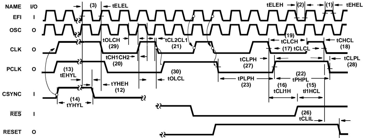
NOTE: All timing measurements are made at 1.5V, unless otherwise noted.
