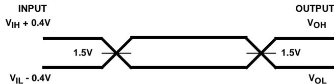
NOTE: Input test signals must switch between  $V_{IL}$  (maximum)  $-0.4\text{V}$  and  $V_{IH}$  (minimum)  $+0.4\text{V}$ .  $\overline{\text{RES}}$  and  $\overline{\text{F/C}}$  must switch between  $0.4\text{V}$  and  $V_{CC} - 0.4\text{V}$ . Input rise and fall times driven at  $1\text{ns/V}$ .  $V_{IL} \leq V_{IL}(\text{max}) - 0.4\text{V}$  for CSYNC pin.  $V_{CC} - 4.5\text{V}$  and  $5.5\text{V}$ .
