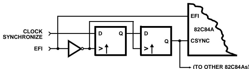
NOTE: If EFI input is used, then crystal input X1 must be tied to  $V_{CC}$  or GND and X2 should be left open. If the crystal inputs are used, then EFI should be tied to  $V_{CC}$  or GND.
