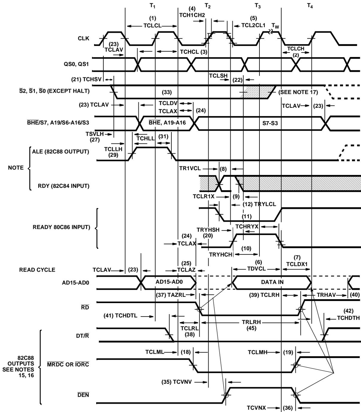
FIGURE 8A. BUS TIMING - MAXIMUM MODE (USING 82C88)
