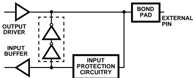
FIGURE 4A. BUS HOLD CIRCUITRY PIN 2-16, 34-39
