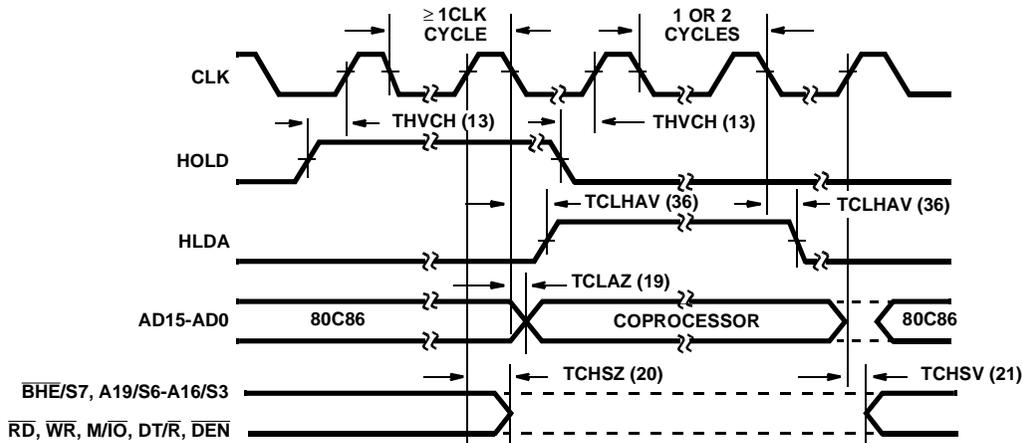
FIGURE 10. HOLD/HOLD ACKNOWLEDGE TIMING (MINIMUM MODE ONLY)
