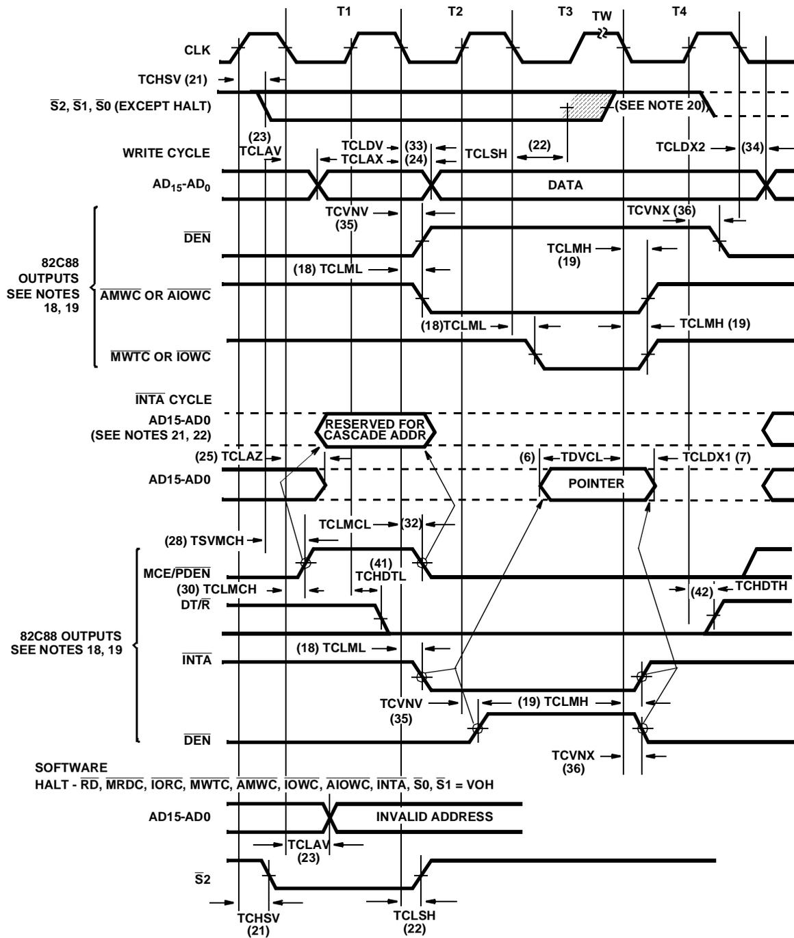
FIGURE 8B. BUS TIMING - MAXIMUM MODE (USING 82C88)
