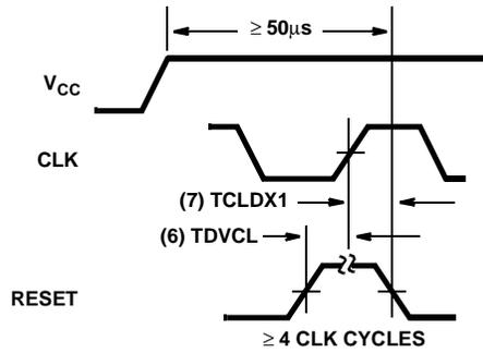
FIGURE 13. RESET TIMING
