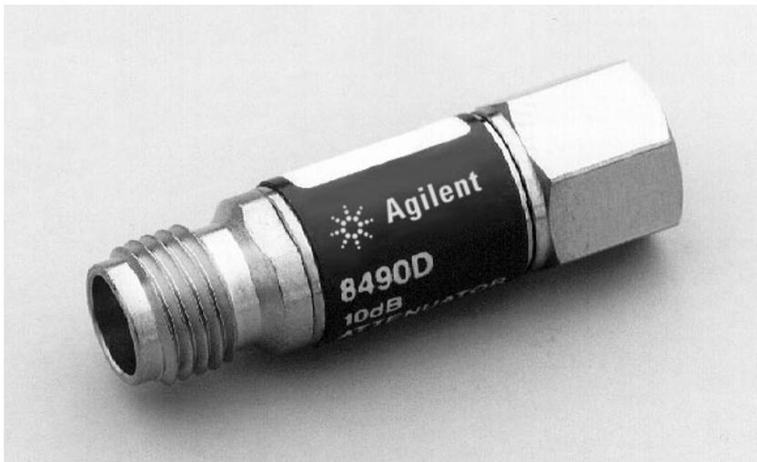
The Agilent Technologies 8490D family is a line of precision fixed coaxial attenuators with performance specified up to 50 GHz. These attenuators use the 2.4 mm coaxial connector, which exhibits excellent performance from dc to 50 GHz. The 8490D family has attenuation values of 3, 6, 10, 20, 30, and 40 dB.
