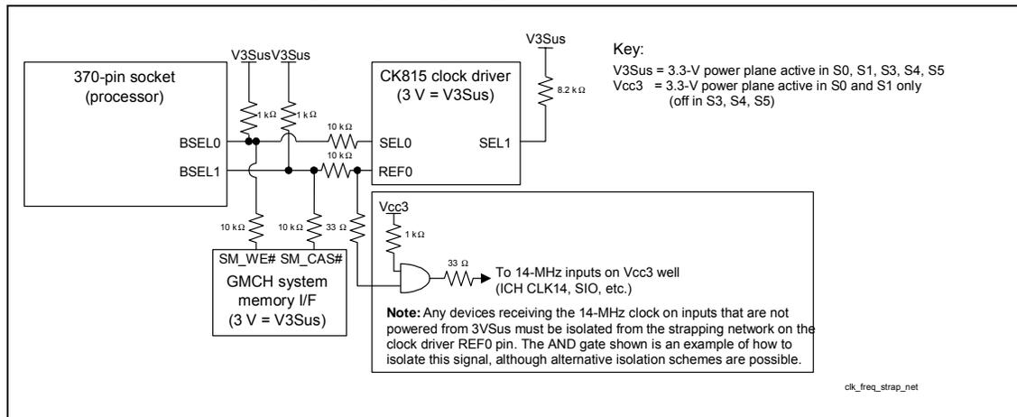
For the platform to come out of a reset properly, clock driver straps powered from the standby supply must be isolated from any logic that powers off in ACPI sleep states.
