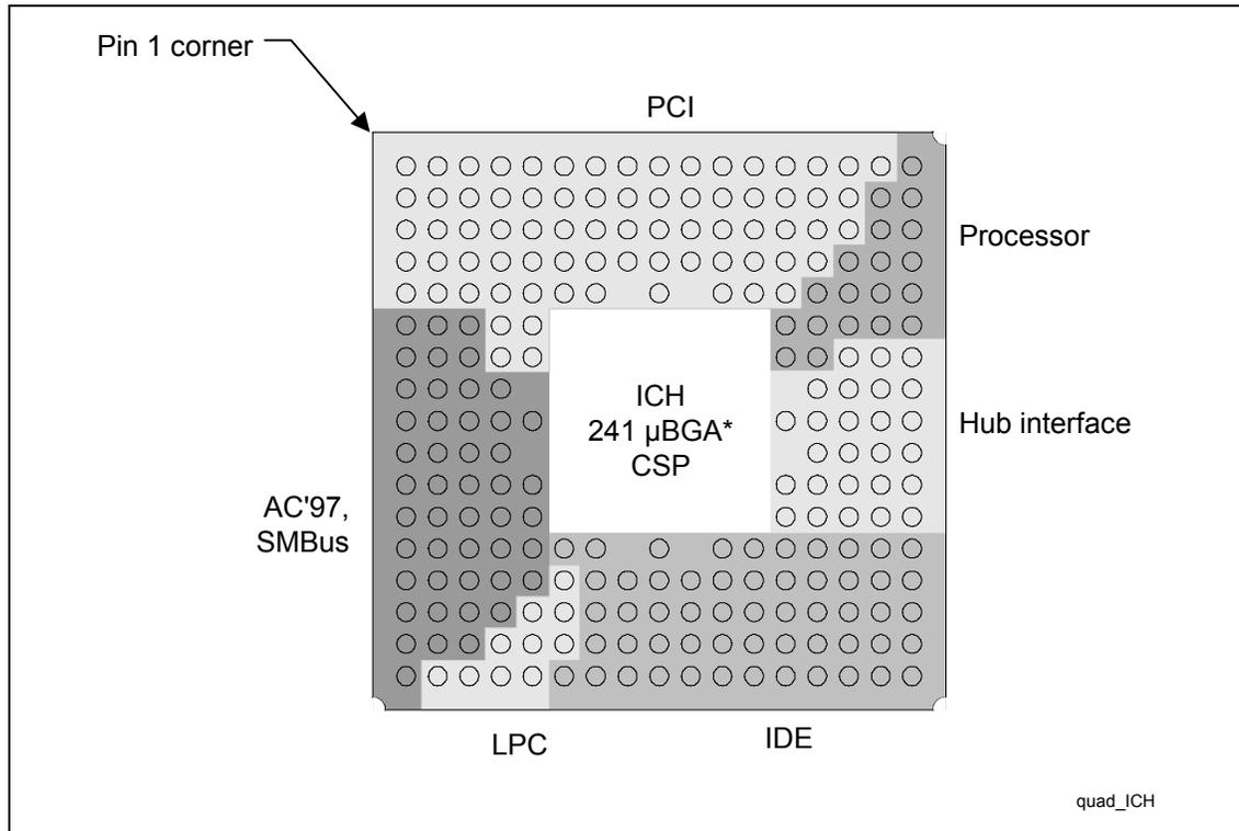
**Note:** This diagram illustrates the relative signal quadrant locations on the ICH ballout. It does not represent the actual ballout. Refer to the *Intel® 82801AA (ICH1) and 82801AB (ICH0) I/O Controller Hub Datasheet* for the actual ballout.
