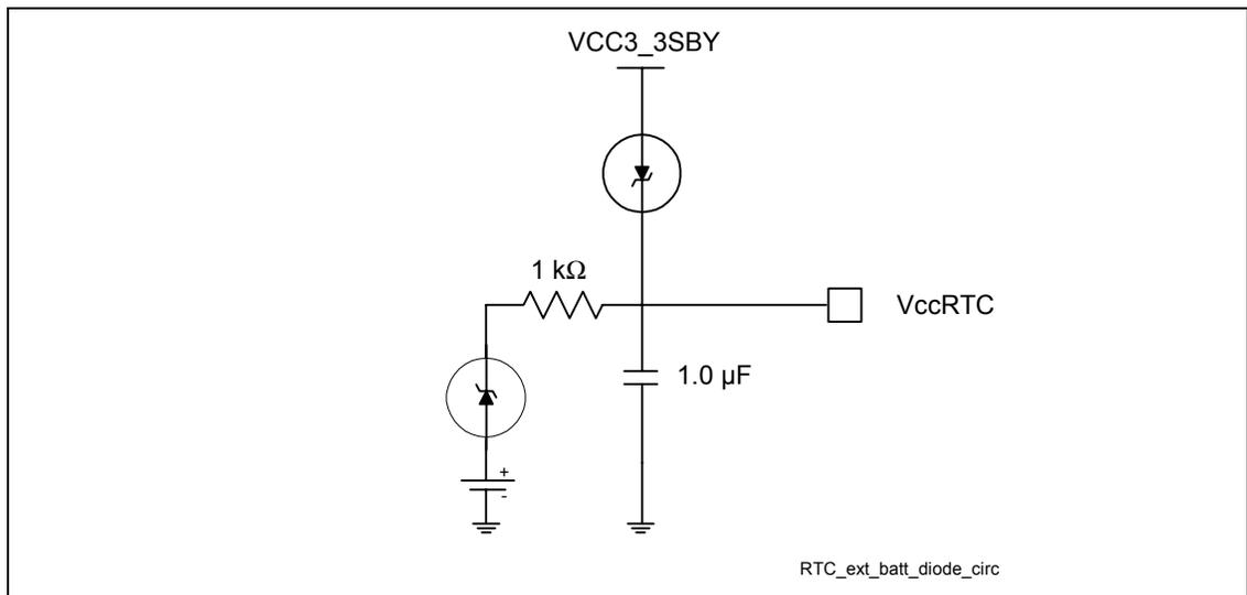
A standby power supply should be used to provide continuous power to the RTC when available, which will significantly increase the RTC battery life and thereby the RTC accuracy.
