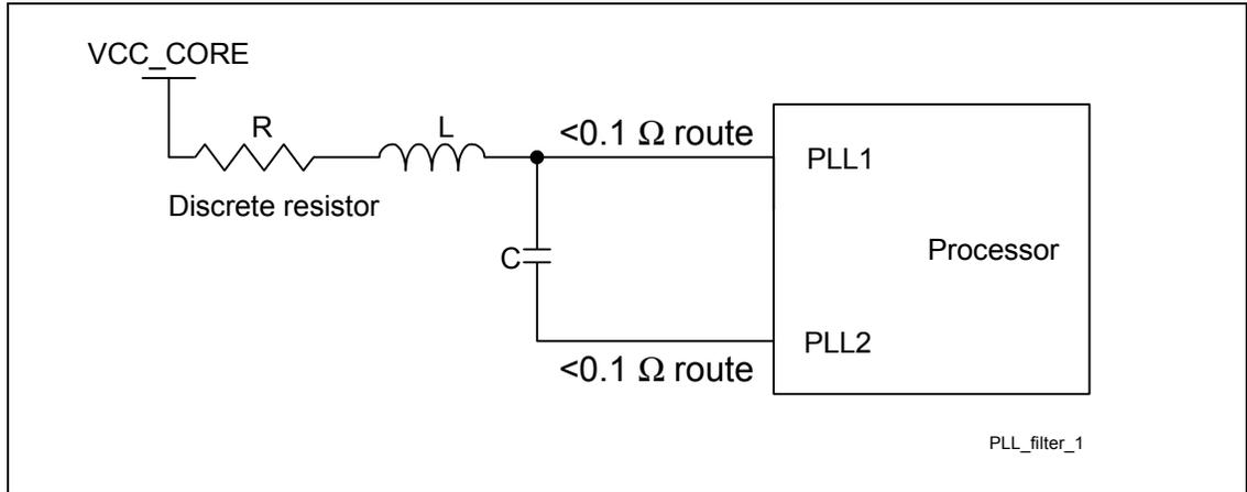
Figure 16. Example PLL Filter Using a Buried Resistor
