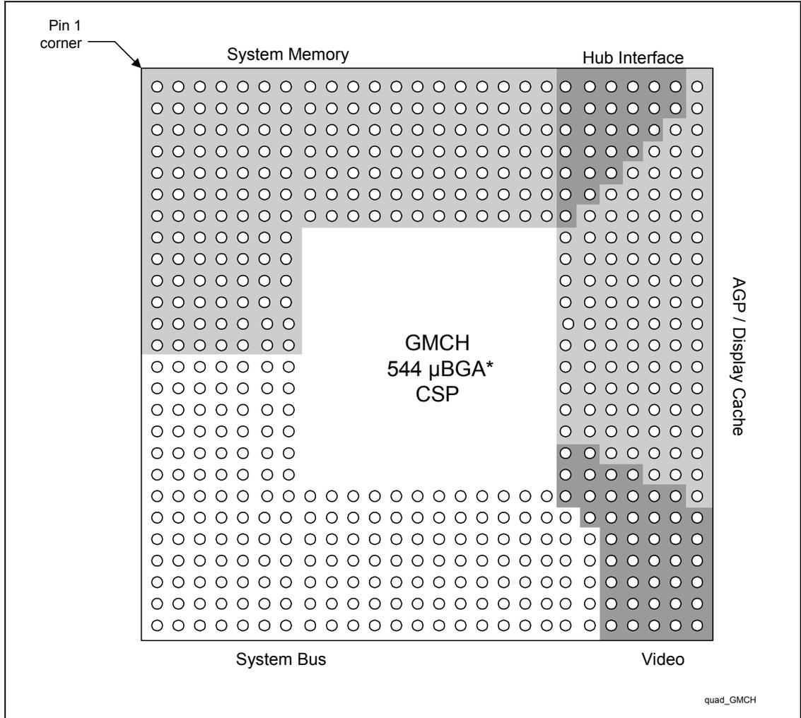
**Note:** This diagram illustrates the relative signal quadrant locations on the Intel 815P chipset MCH ballout. It does not represent the actual ballout. Refer to the *Intel® 815 Chipset Family: 82815E and 82815P Memory Controller Hub (MCH) Datasheet* for the actual ballout.
