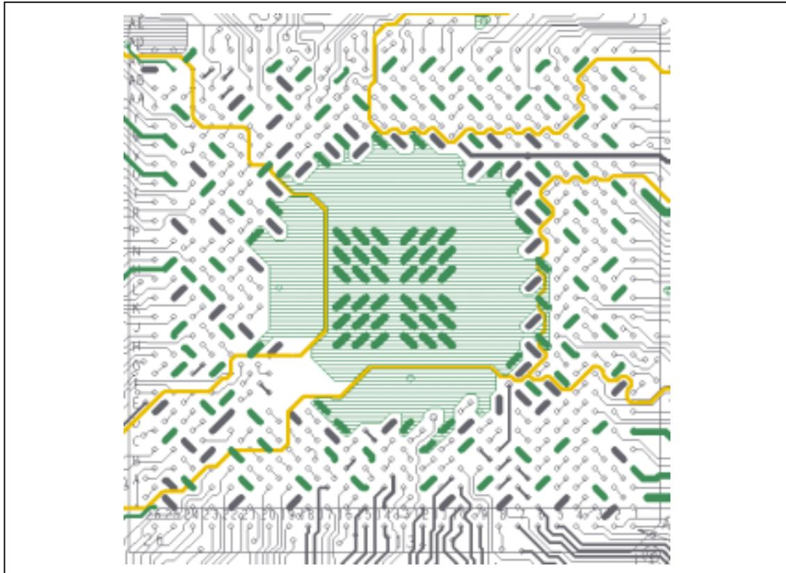
The filled region in the middle of the MCH indicates a ground plate (on layer 1 if the power plane is on layer 2 or on layer 4 if the power layer is on layer 3).
