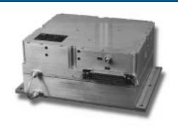
This indirect synthesizer provides both wide bandwidth and moderate switching speeds in a package volume less than 155 cubic inches. The 625 kHz resolution is achieved using a dual loop architecture.
