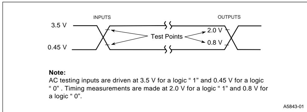
Figure 16. Float Test Conditions
