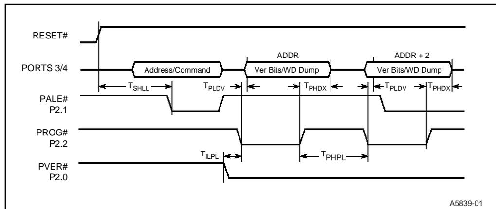
**Figure 19. Slave Programming Mode Timing in Data Program Mode with Repeated Program Pulse and Auto Increment**
