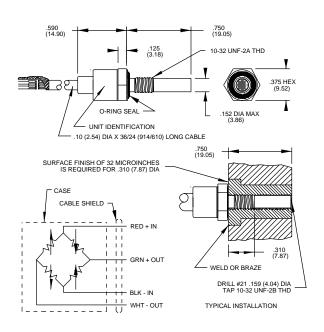
STANDARD TOLERANCE INCHES (MILLIMETERS) .XX = +/- .03 (.X = +/- .8) .XXX = +/- .010 (.XX = +/- .25)
