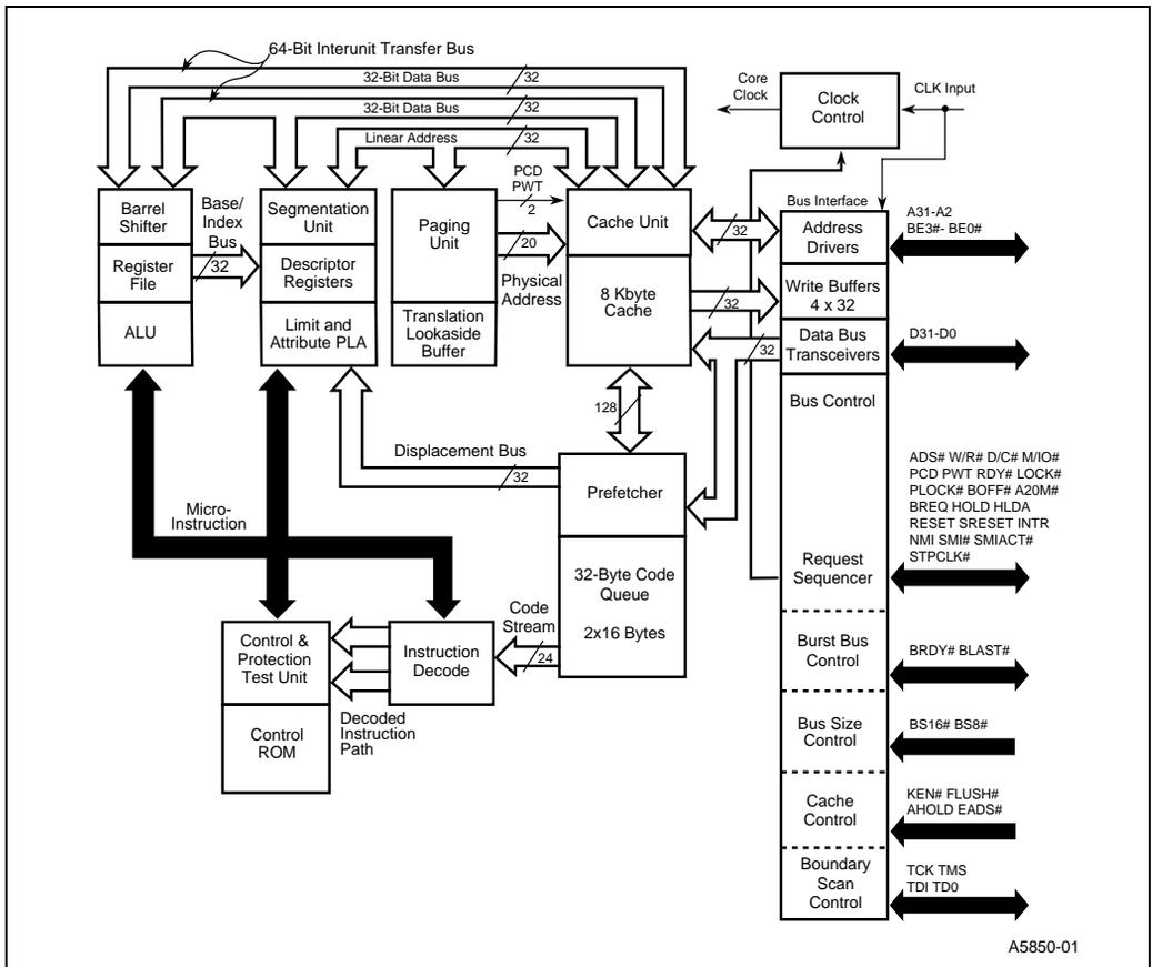
Figure 1. Embedded Ultra-Low Power Intel486™ SX Processor Block Diagram
