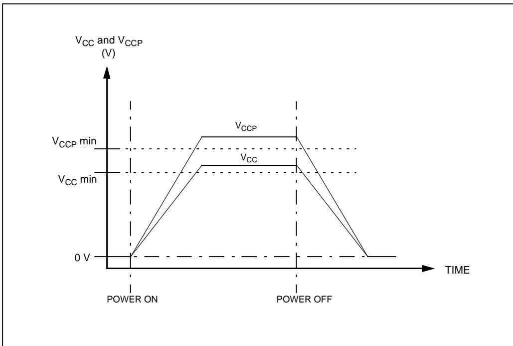
Figure 3. Example of Supply Voltage Power Sequence
