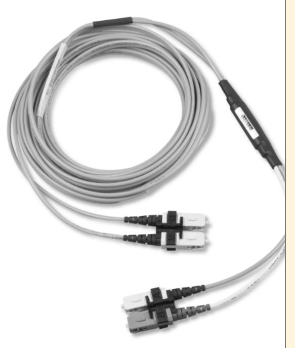
To optimize long-wave (1300 nm) multimode Gigabit Ethernet (GbE) applications, Storm Products—Fiber Optics offers a mode-conditioning patch cord. This patch cord functions the same as a standard patch cord but contains an offset singlemode-to-multimode fiber connection point. The offset encasement is both rugged and low profile.
