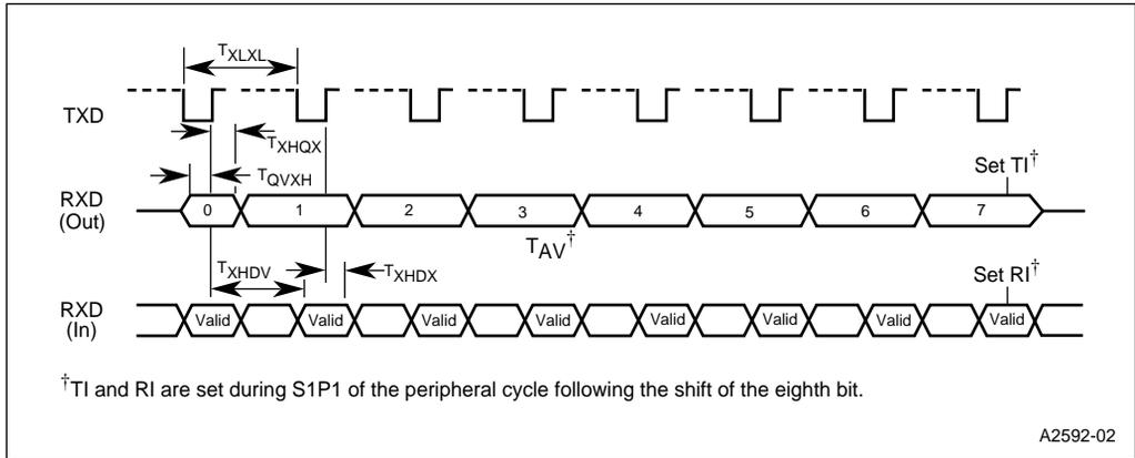
**Figure 11. Serial Port Waveform — Shift Register Mode**
