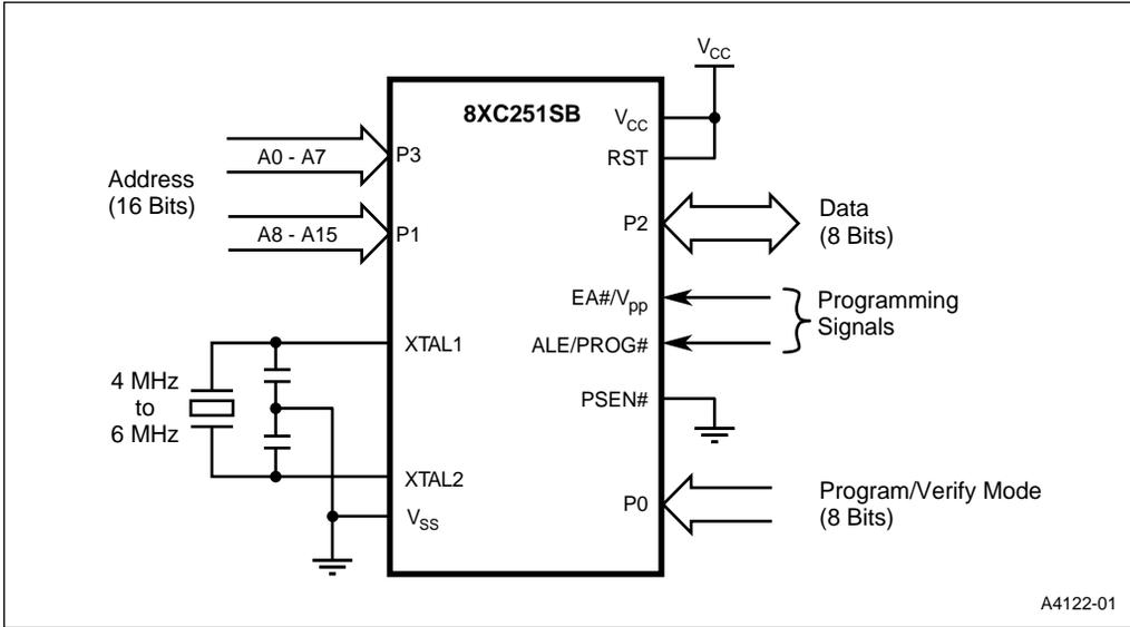
Figure 15. Setup for Programming and Verifying Nonvolatile Memory
