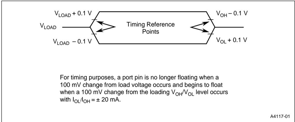
**Figure 14. Float Waveforms**
