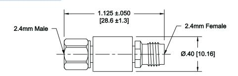
Note: Dimensions in Brackets are Expressed in Millimeters and are for Reference Only. Overall lengths are with coupling nuts biased forward (install length)
