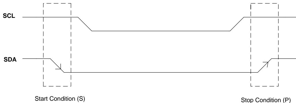
Figure 1. I 2 C Start and Stop Condition
