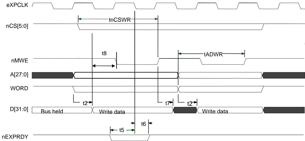
Notes: 1.  $t_{nCSWR} = 35 \text{ nsec}$  at 36.864 MHz, 70 ns at 18.432 MHz
