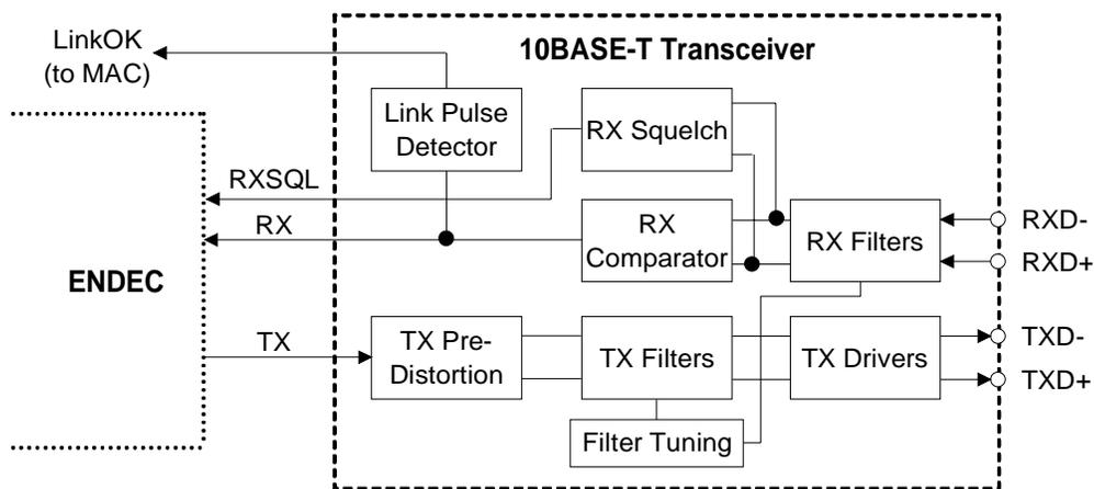
**Figure 17. 10BASE-T Transceiver**
