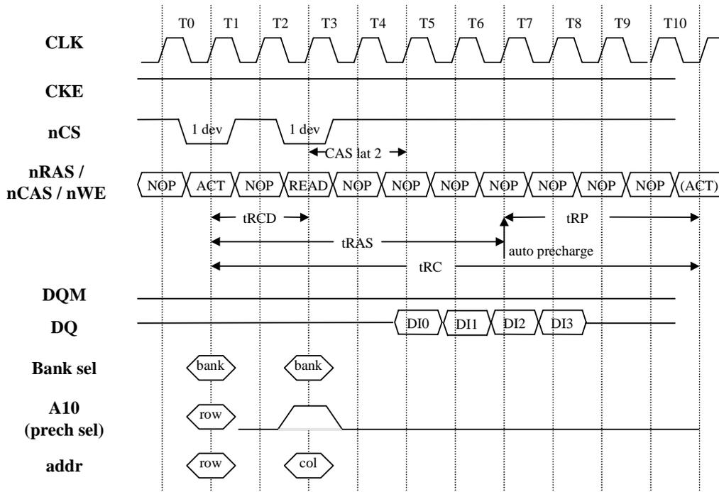
1. tRCD (delay time ACT to READ/WRITE command) = 30 ns or 2 cycles at 36 MHz.
