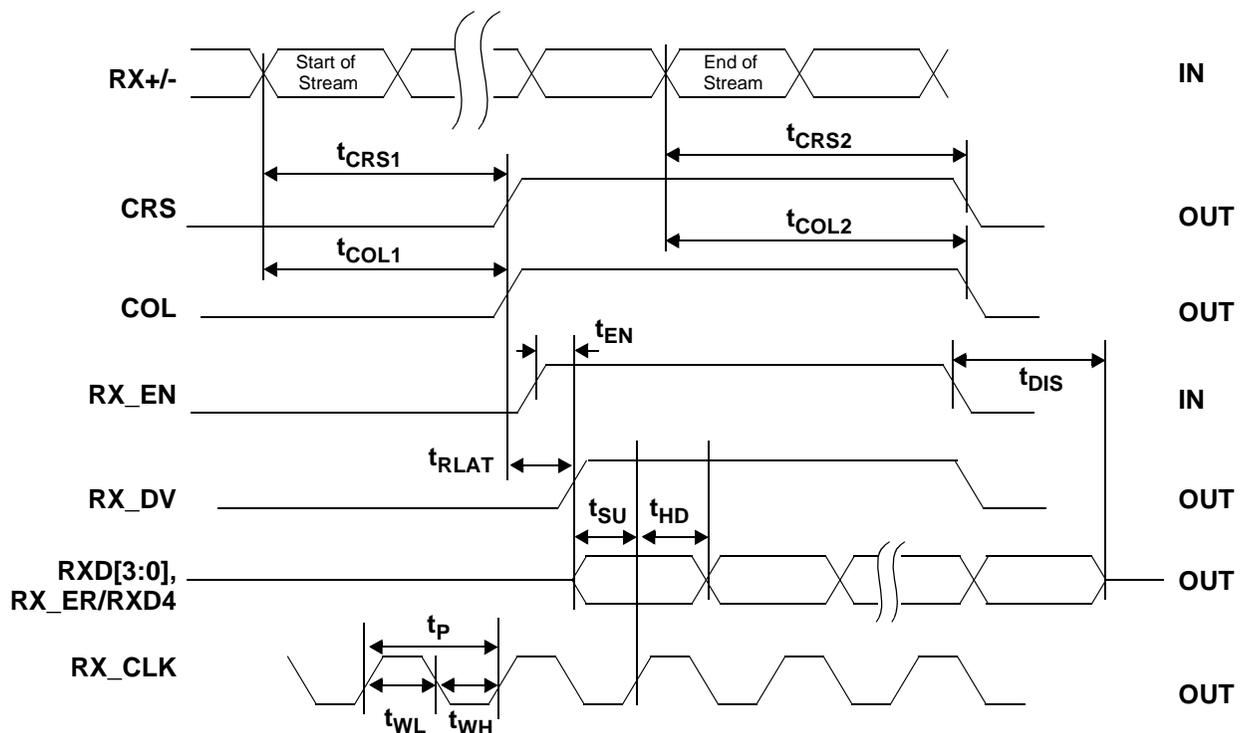
**100BASE-TX MII RECEIVE TIMING - 5B BYPASS ALIGN MODE**
