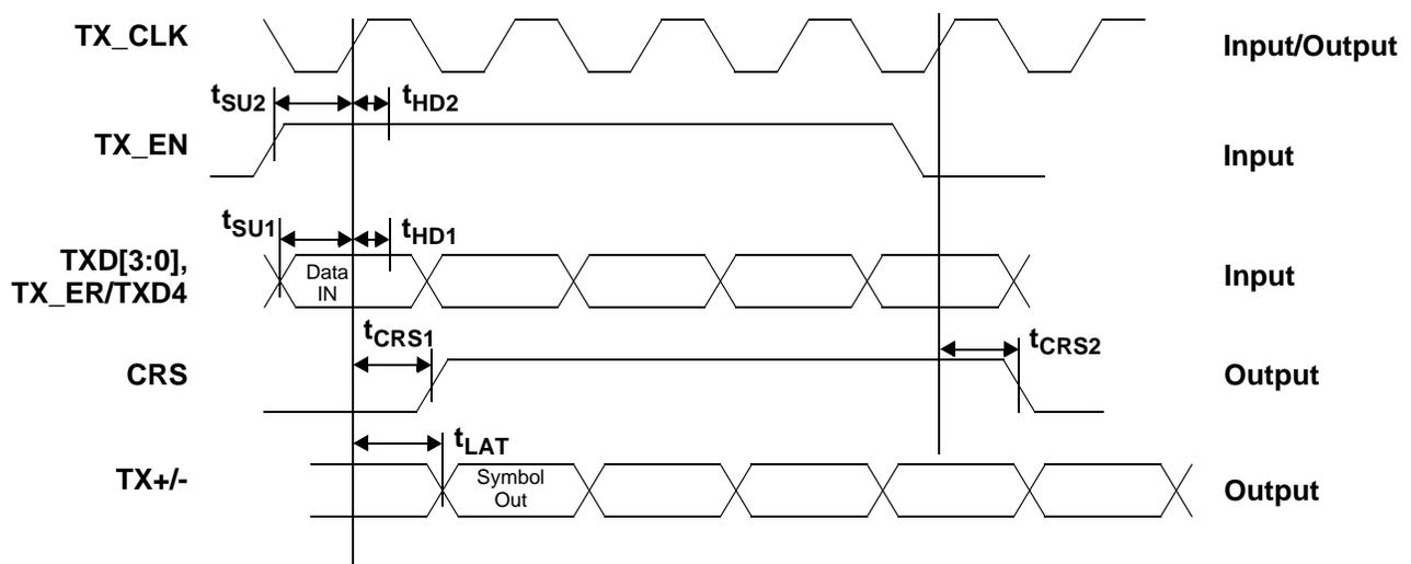
**100BASE-TX MII TRANSMIT TIMING - 5B BYPASS ALIGN MODE**
