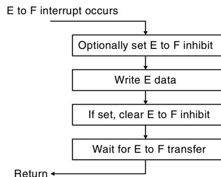
Figure 15. Flowchart for Writing the E Buffer
