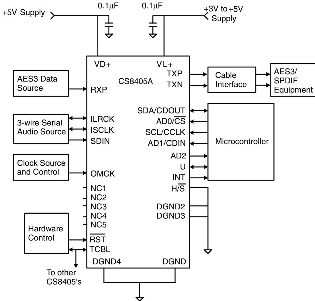
**Figure 5. Recommended Connection Diagram for Software Mode**
