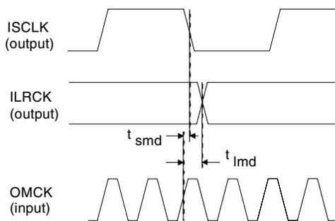
**Figure 1. Audio Port Master Mode Timing**
