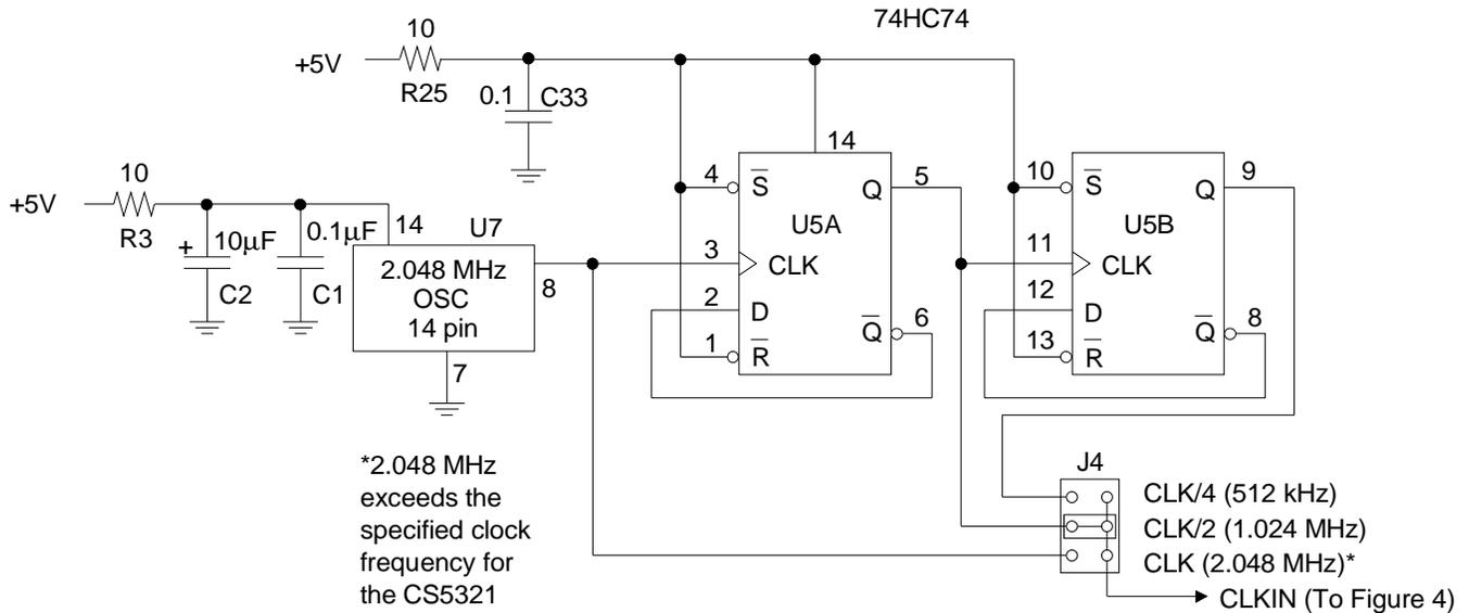
**Figure 3. Oscillator / Divider**
