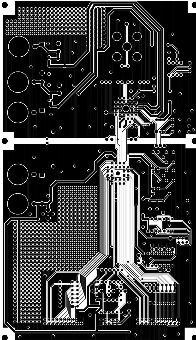
Figure 9. CDB5321 (Rev. C) Solder Side Layer (Not to Scale)
