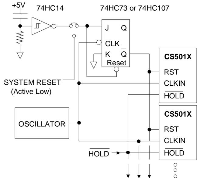
**Figure 4. Controlled Reset for Synchronizatoiin of Multiple Converters**
