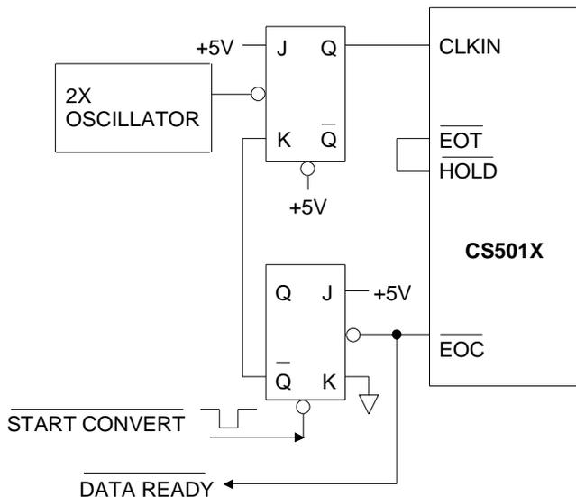
**Figure 3. Coarse Charge Jamming with "StartConvert" Control**
