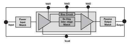
Single control bias setting for low Idq and 40%PAE at Pout = 28.5 dBm
