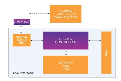
The Cirrus CS22230 Wireless Mini PCI Controller incorporates the IEEE 802.11b media access controller (MAC) to enable Wi-Fi compliant wireless network devices providing industry-wide interoperability. In addition, the CS22230 supports our multimedia and quality of service (QoS) extensions to distribute entertainment content wirelessly throughout the home network – with unparalleled performance.
