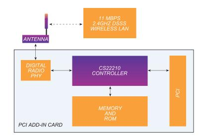
The Cirrus CS22210 Wireless PCI/USB Controller incorporates the IEEE 802.11b media access controller (MAC) to enable Wi-Fi compliant wireless network devices providing industry-wide interoperability. In addition, the CS22210 supports our multimedia and quality of service (QoS) extensions to distribute entertainment content wirelessly throughout the home network – with unparalleled performance.
