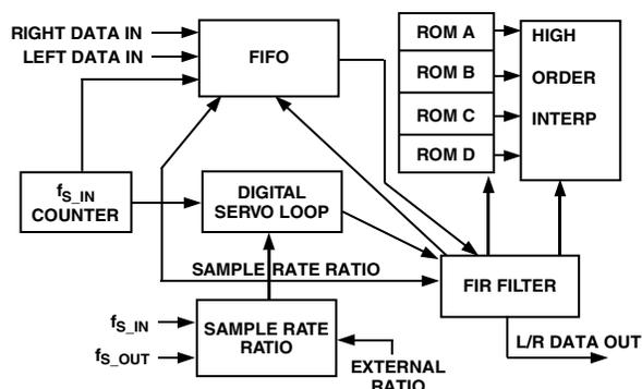
Figure 7. Architecture of the Sample Rate Converter
