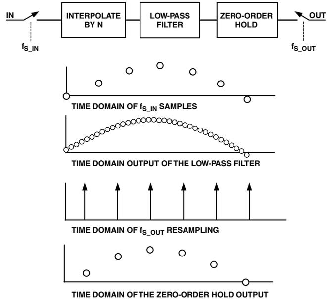
Figure 5. Time Domain of the Interpolation and Resampling
