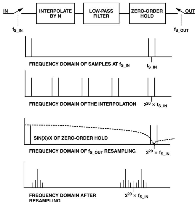
Figure 6. Frequency Domain of the Interpolation and Resampling
