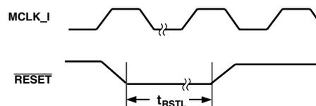
Figure 2.  $\overline{\text{RESET}}$  Timing
