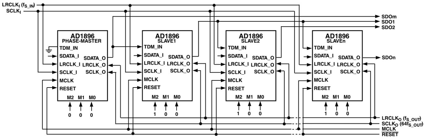
Figure 13. Typical Configuration for Matched Phase Mode Operation
