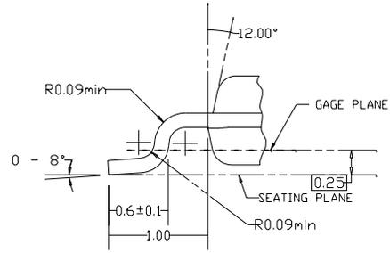
DIMENSIONS ARE IN MILLIMETERS
