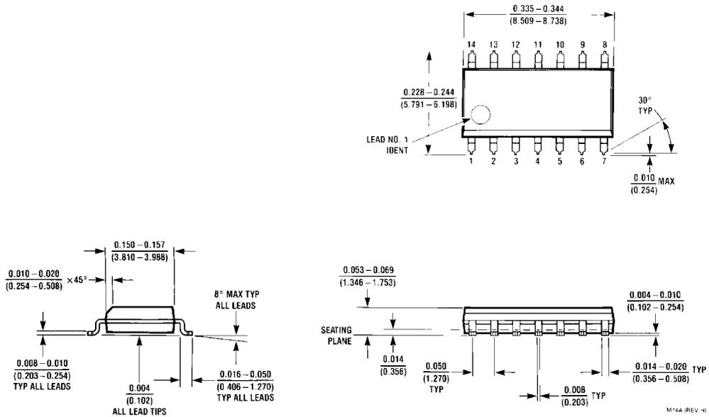
**14-Lead Small Outline Integrated Circuit (SOIC), JEDEC MS-012, 0.150" Narrow
