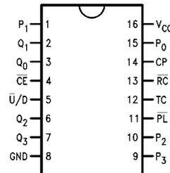
74F191 Up/Down Binary Counter with Preset and Ripple Clock
