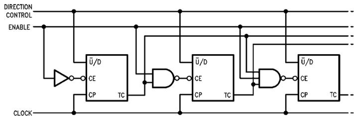
FIGURE 3. Synchronous n-Stage Counter with Gated Carry/Borrow
