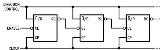
FIGURE 2. Synchronous n-Stage Counter Using Ripple Carry/Borrow
