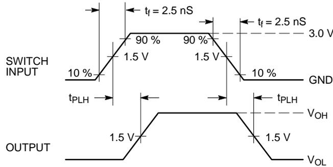
**Figure 4. Propagation Delays**
