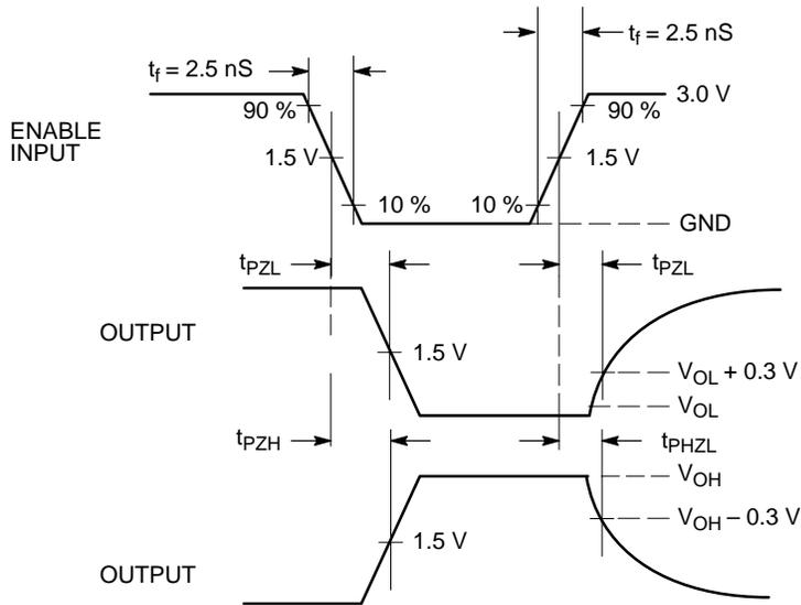
**Figure 5. Enable/Disable Delays**
