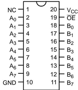
Figure 1. 20-Lead Pinout
