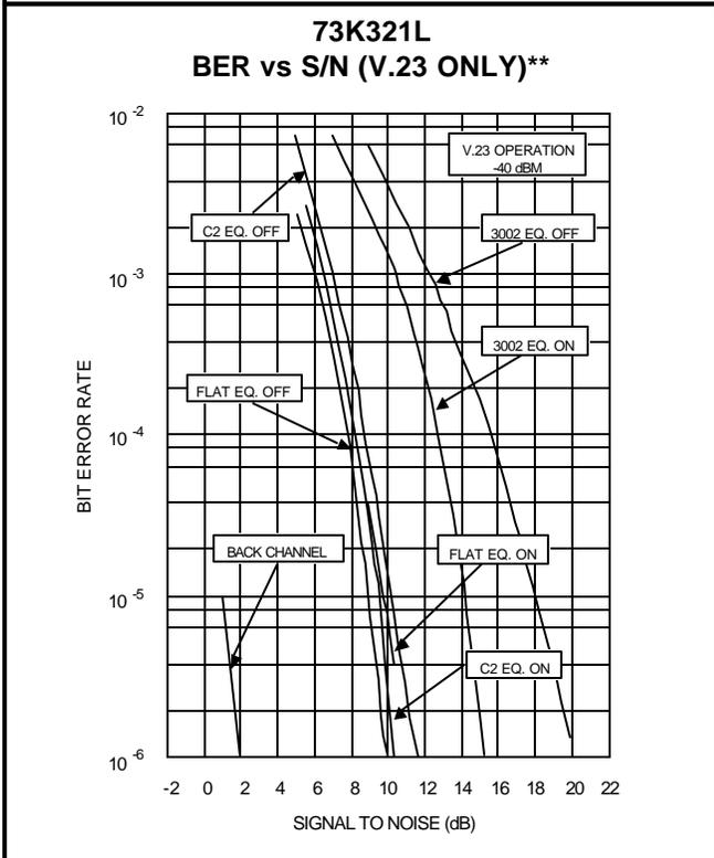
\* = "EQ On" Indicates bit CR1 D4 is set for additional phase equalization.
