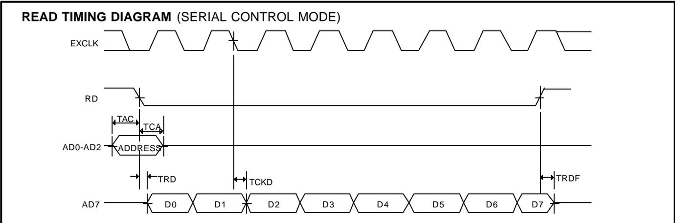
Note: EXCLK must be low to read D0 after  $\overline{RD}$  is asserted
