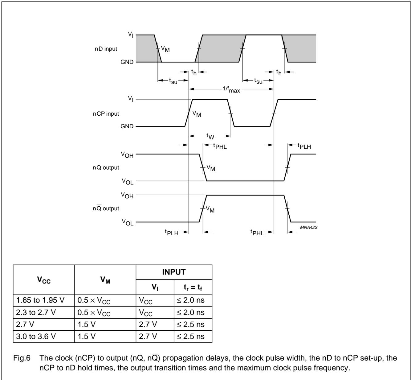
Fig.6 The clock (nCP) to output (nQ, nQ-bar) propagation delays, the clock pulse width, the nD to nCP set-up, the nCP to nD hold times, the output transition times and the maximum clock pulse frequency.
