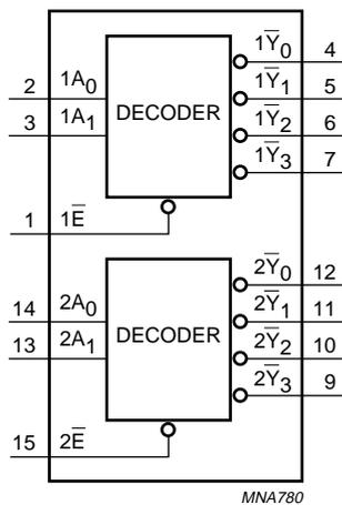
Fig.5 Functional diagram.
