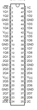
A buffered output-enable  $(\overline{OE})$  input can be used to place the outputs in either a normal logic state (high or low logic levels) or the high-impedance state. In the high-impedance state, the outputs neither load nor drive the bus lines significantly. The high-impedance state and the increased drive provide the capability to drive bus lines in a bus-organized system without need for interface or pullup components.
