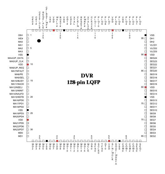
Figure 3.1 W9980D Pin configuration
