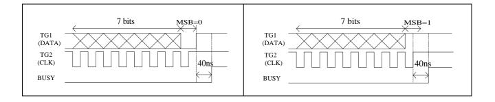
To place the W583xxx in CPU mode, program the code according to the following example.
