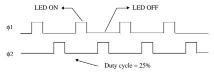
The  $\phi1$  clock is applied to LED1 output pin definitely. For flashing synchronously of the LEDs, the  $\phi1$  clock is also connected to LED2. For flashing alternately, the  $\phi2$  clock is connected to LED2. In other words, LED outputs flash synchronously with the  $\phi1$  clock or flash alternately in two groups, one is LED1 with  $\phi1$  and the other is LED2 with  $\phi2$ .
