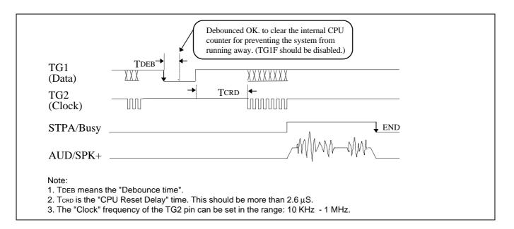
Busy signal will output "high" after the end of transmission. The rising timing of Busy signal is dependent on the MSB of data output on TG1(Data) pin. If MSB is "1", Busy will rise after the last rising edge of TG2(Clock) pin. If MSB is "0", Busy will rise after the rising edge that TG1(Data) returns to high.
