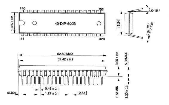
NOTE: Dimensions are in millimeters.
