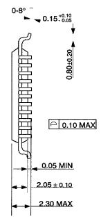
NOTE: Dimensions are in millimeters.
