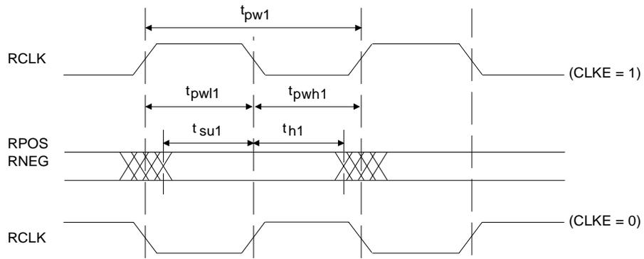
**Figure 2. Recovered Clock and Data Switching Characteristics**
