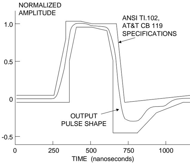
**Figure 6. Typical Pulse Shape at DSX-1 Cross Connect**
