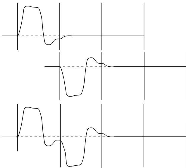
**Figure 14. Example of Summing of Waveforms**
