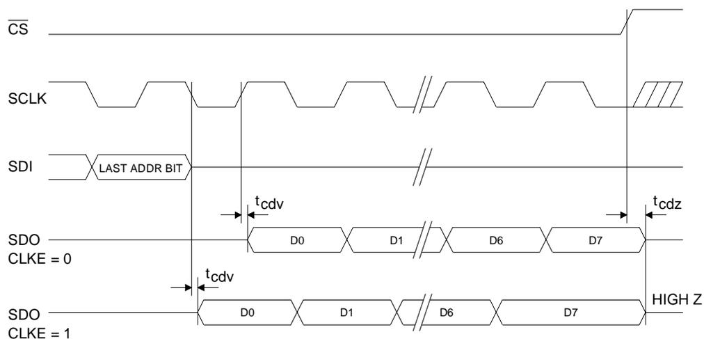
**Figure 5. Serial Port Read Timing Diagram**
