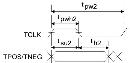
**Figure 3. Transmit Clock and Data Switching Characteristics**
