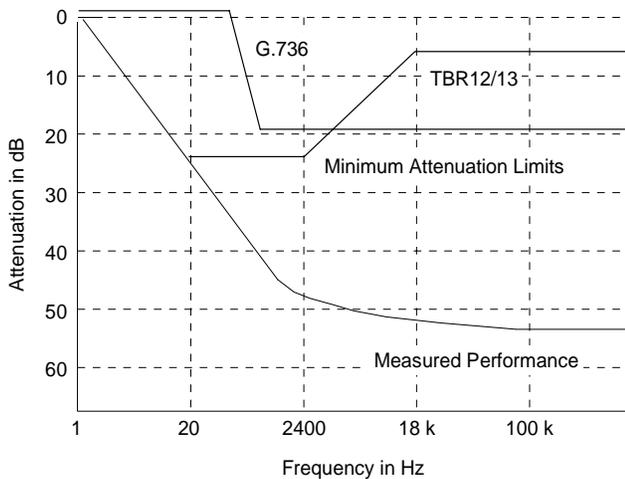
**Figure 11. Typical Jitter Transfer Function - E1**
