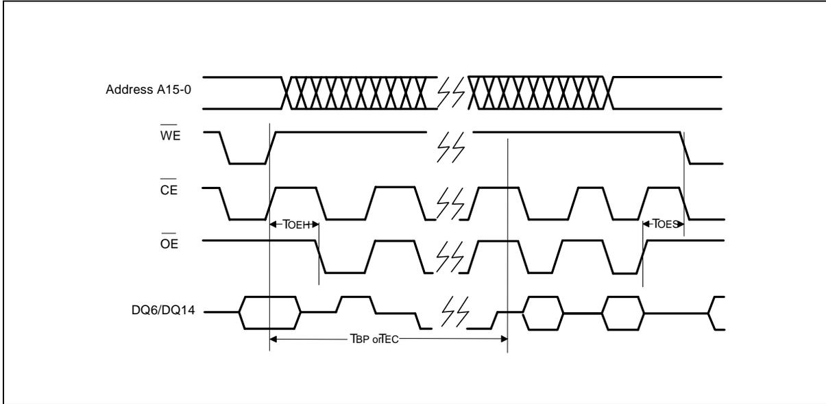
**Boot Block Lockout Enable Timing Diagram**
