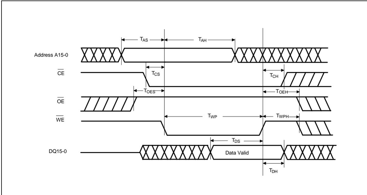
**$\overline{\text{CE}}$  Controlled Command Write Cycle Timing Diagram**
