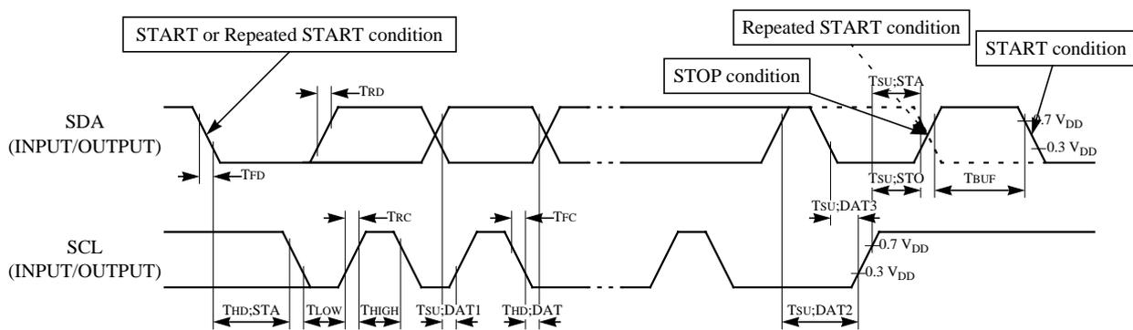
**Figure 26. I<sup>2</sup>C Waveforms**
