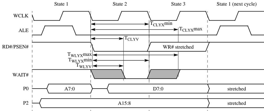
Figure 23. Real-time Synchronous Wait State: Data Write
