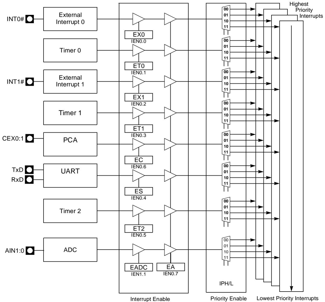
Each of the interrupt sources can be individually enabled or disabled by setting or clearing a bit in the Interrupt Enable register. This register also contains a global disable bit which must be cleared to disable all the interrupts at the same time.
