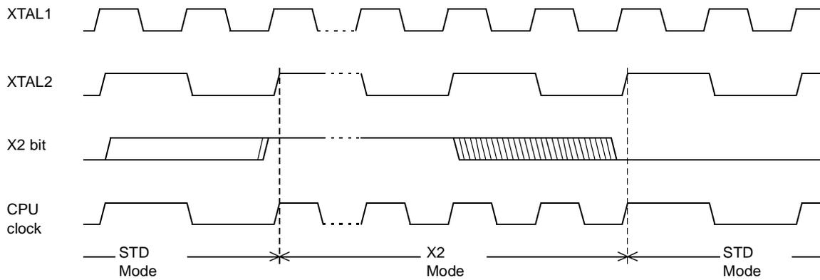
Note: In order to prevent any incorrect operation while operating in the X2 mode, users must be aware that all peripherals using the clock frequency as a time reference (UART, timers...) will have their time reference divided by two. For example a free running timer generating an interrupt every 20 ms will then generate an interrupt every 10 ms. A UART with a 4800 baud rate will have a 9600 baud rate.
