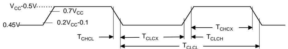
**AC Testing Input/Output Waveforms**
