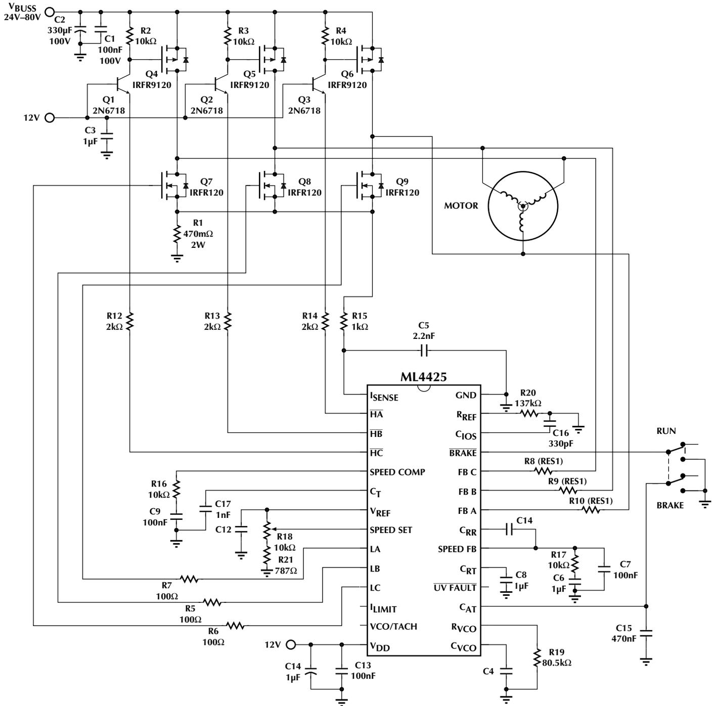
Figure 11. Driving Lower Voltage Motors (12 to 80V)
