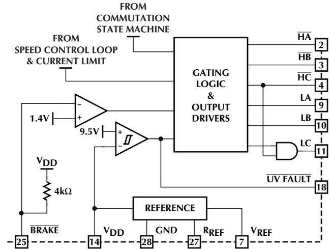
Figure 10. Cross Conduction, Brake, and UVLO Circuits
