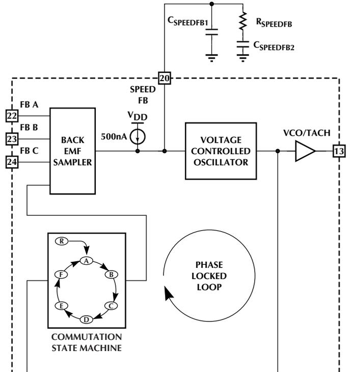
Figure 7. Back EMF Commutation Phase Locked Loop
