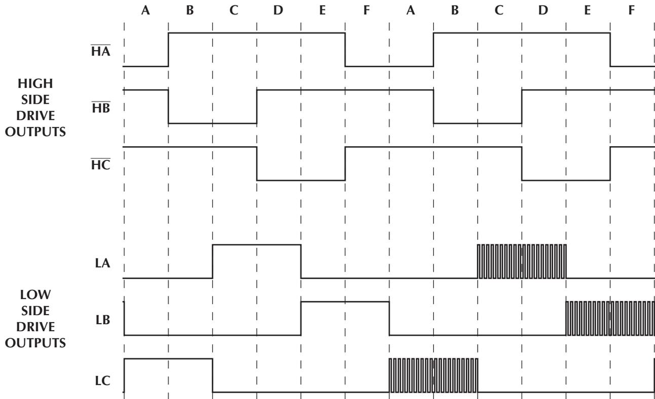
**Figure 4. Output Commutation Sequence Timing Diagram**
