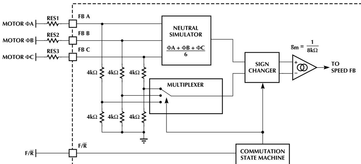
Figure 6. Back EMF Sampler Detailed Block Diagram
