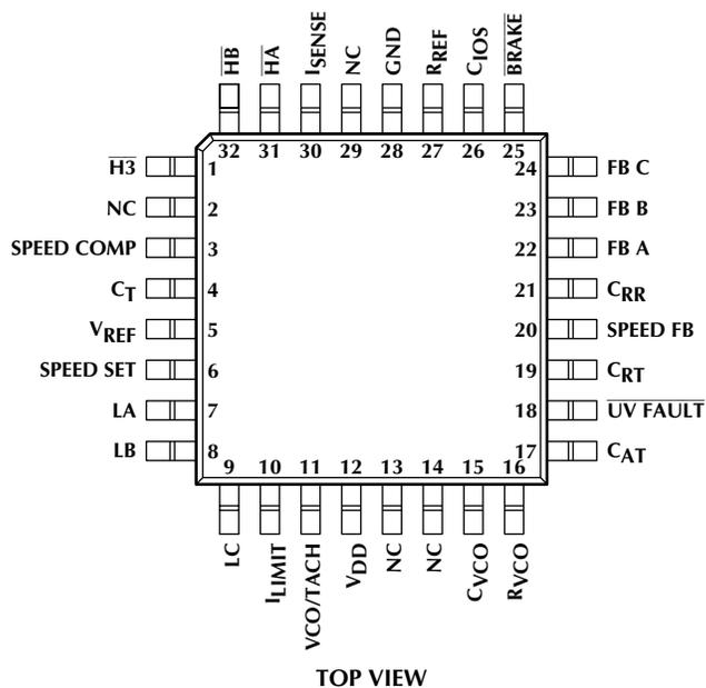
**PIN DESCRIPTION** (Pin number in parenthesis is for TQFP package)
