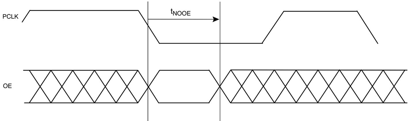
Note: OE must not change during TNOOE after the PCLK falls. This is to ensure that the output drivers of the data is not driving current, to reduce the noise level on the power supply.
