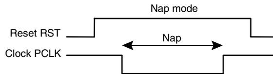
In Nap Mode, all internal transistors are in shut mode. Only leakage current is drained in power supply, generally less than the tested value.
