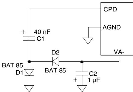
**Figure 5. Generating VA- with a Charge Pump**
