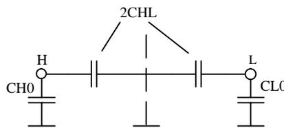
Capacitance H:  $CH_{gnd} = CH0 + 2 CHL \leq 200 \text{ pF/m}$
