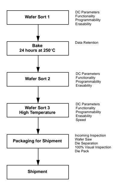
Figure 1. AMD KGD Product Test Flow
