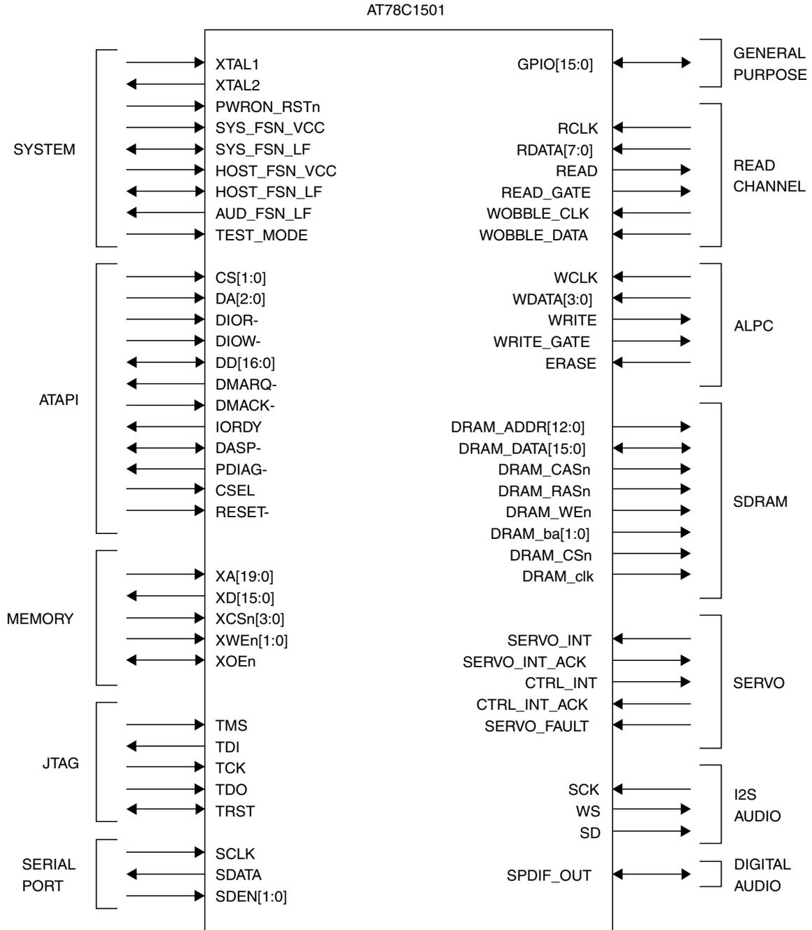
Figure 4. AT78C1501 Block Diagram
