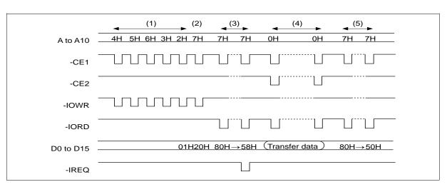
2. Sector write: 1 sector write procedure after the card configured I/O interface is shown as follows.
