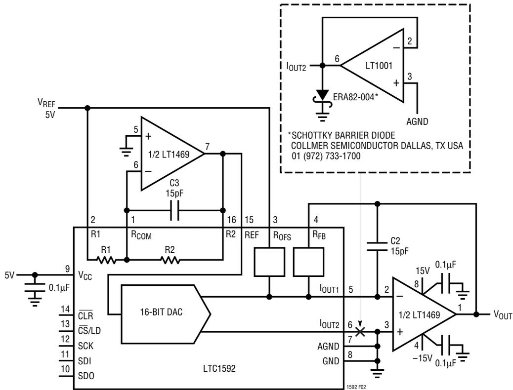
Figure 2. Driving  $I_{OUT2}$  from AGND with a Force/Sense Amplifier
