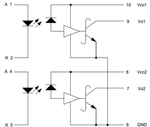
NOTE: A. .01 TO 0.1 uF BYPASS CAPACITOR
