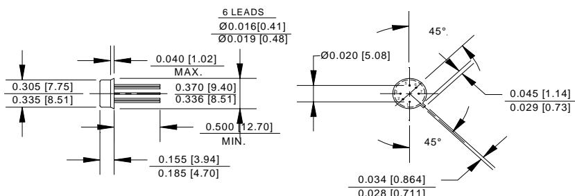
NOTE: ALL LINEAR DIMENSIONS ARE IN INCHES (MILLIMETERS)
